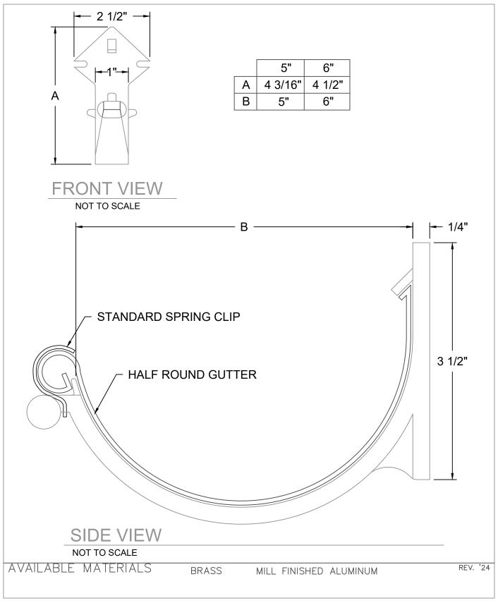
IN AREAS SUBJECT TO SNOW SLIDE, COORDINATE THE FRONT EDGE ELEVATION OF GUTTERS WITH ROOF SLOPE LINE.
