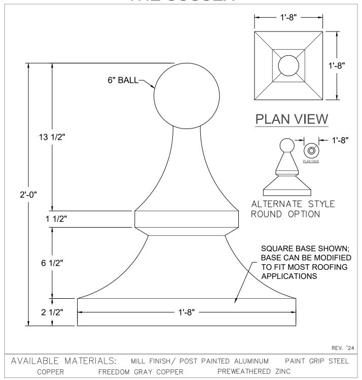
WEIGHT: VARIES DEPENDING ON ROOF CONDITION, ROOF SLOPE AND MATERIAL SEAL THE MOUNTING BRACKET (PROVIDED) TO THE ROOF SURFACE FOR A WATERTIGHT INSTALLATION. SET SPIRE BASE OVER MOUNTING BRACKET AND ATTACH USING FASTENERS PROVIDED. SPECIFY ROOF SLOPE FOR BRACKETS. **INSTALLATION:**
